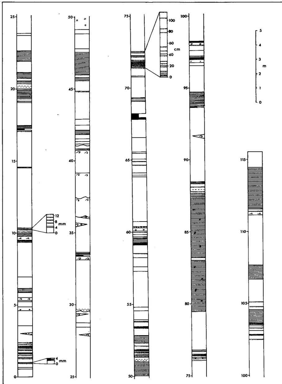
**Fig. 3.11:** Sedimentary log of the Rhino Wash section. Plate 8.B is a photograph of this section. Note the very thinly bedded facies D<sub>1</sub> units interbedded with facies B<sub>1</sub>.
