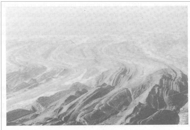
**Plate 1.B:** Oblique aerial photograph of three Ramsay type 2c interference folds caused by northwest-southeast shortening of the tight north-south  $F_1$  folds. View looking north in the west of the area.
